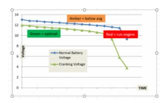
Redtail have studied the battery voltages required to start a car reliably and reprogrammed their black boxes in situ to send battery status information to their DataWarehouse. In turn this information is translated into alerts that can be pushed out to vehicle owners by email or SMS.
